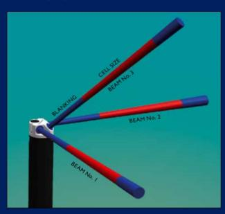
The current meter had a sidelooking sensor head transmitting and receiving sound along three narrow acoustic beams.
